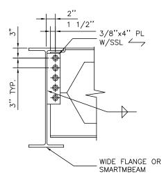
Beam-to-Beam Shear Tab Conx.
