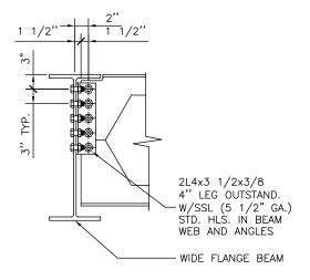
Beam-to-Beam Bolted-Bolted Clip Ang. Conx.
