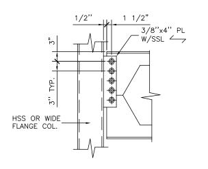
Beam-to-Column Shear Tab Conx.
