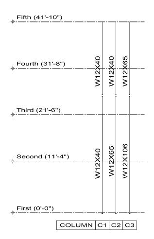
1) Boxes indicate lateral force resisting (Chevron braced) frames. NO special base plate detail is assumed for the columns.
