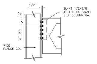
Beam-to-Column Bolted-Welded Clip Ang. Conx.
